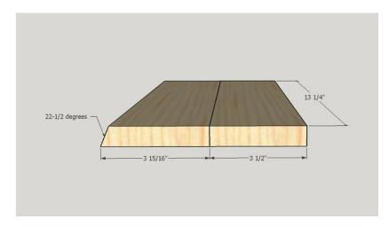
Place the step flush with the front of the legs and mark the angle at the back of the legs. Using a table saw or circular saw, cut a 22.5-degree angle at this mark. Clamp in position. Attach to the cleats using 2" wood screws and attach to the front rail using 1-1/2" pocket screws.
